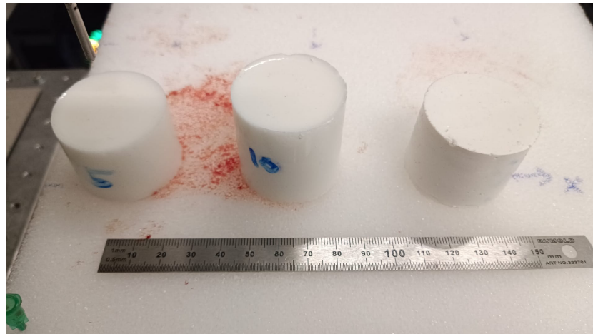
Fig. 3: A photo of our custom plastisol phantoms, sorted by elasticity. From left to right, they correspond evenly to G5-G15 of table 2.2.
