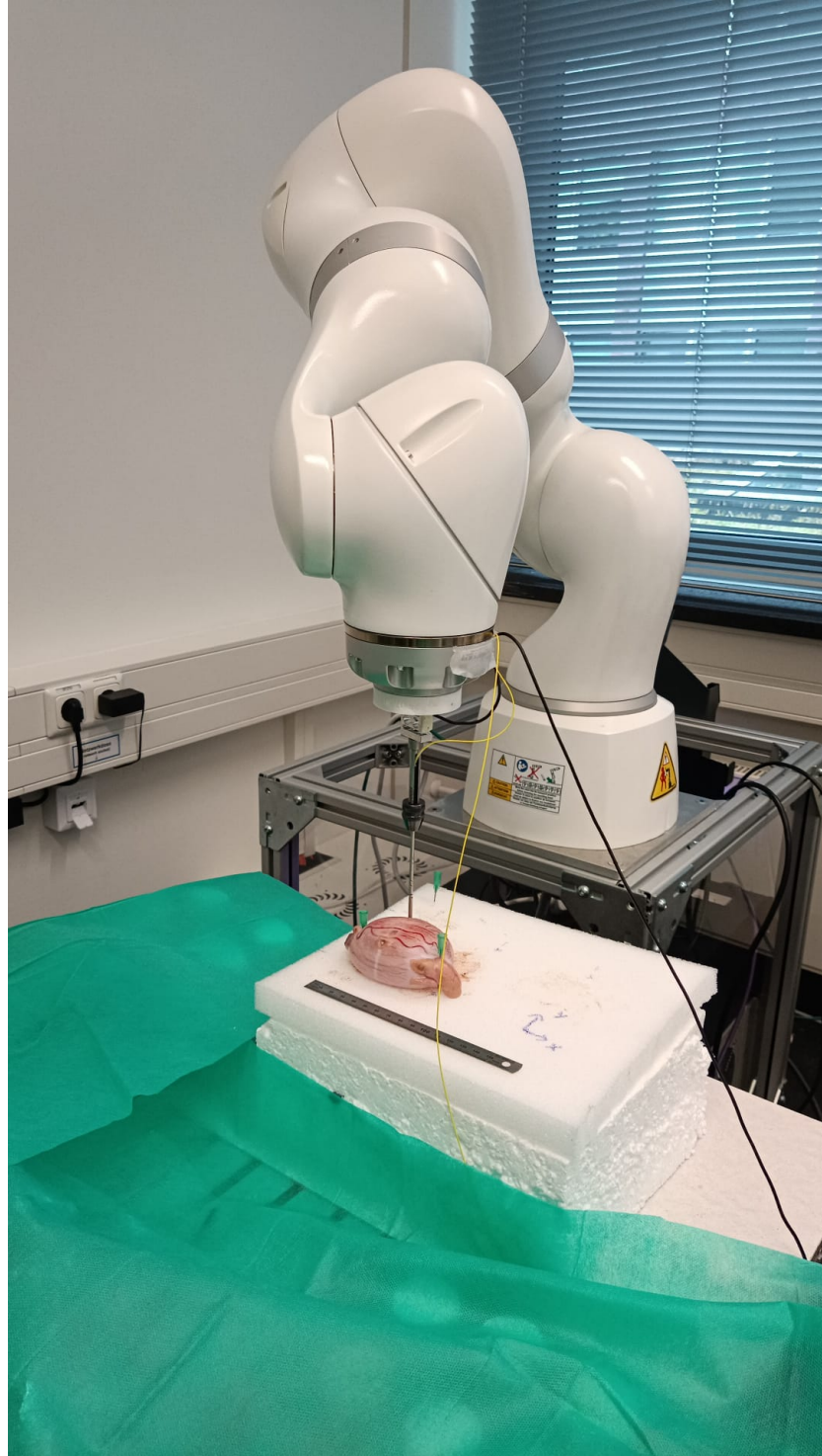
Fig. 5: A photo of our full setup in our laboratory at MTEC. We can see the KUKA robot arm standing on a scaffold with its computer below. The needle is mounted as the end-effector. An OCT fiber (yellow) leads to the OCT device (not seen) and a black cable leads from the force sensor at the needle shaft to its receiver (not seen). A lamb testicle lays fixated on a thinner styrofoam plate, which can be replaced for sanitary reasons. Below, there is a thicker styrofoam plate for leverage. A large green cloth covers the rest of the table.
